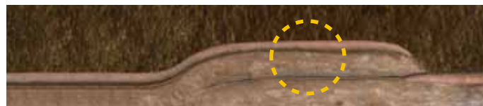
Bentonite granules within BentoShield swell and form monolithic sealing layer in overlap zones.
